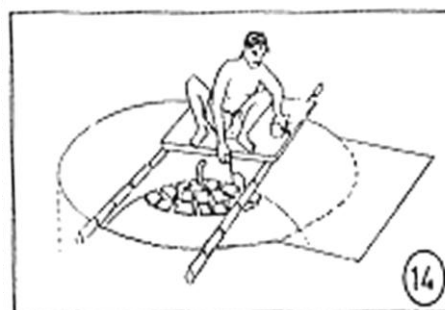
Closing of dome with bricks
