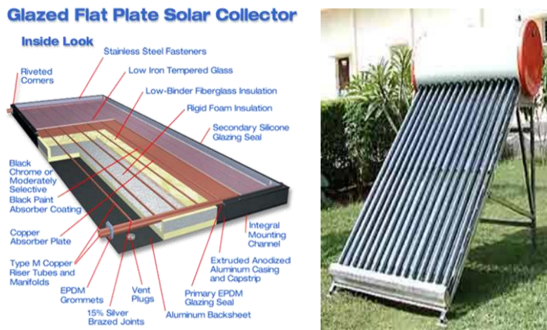
Fig.3 .Flat Plate liquid collector
