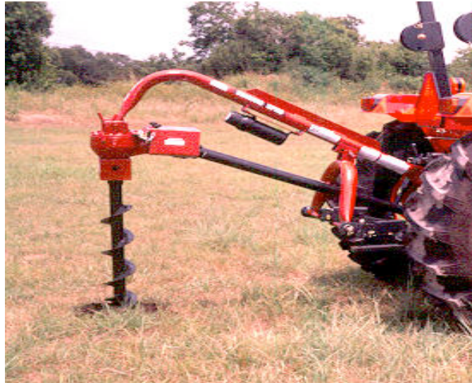
Tractor operated Post hole digger- gear drive
