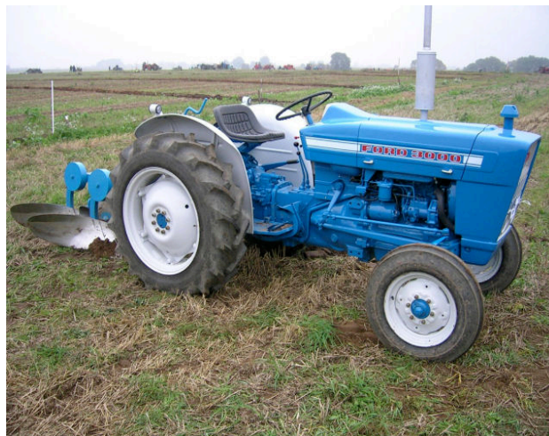
Tractor with two bottom mouldboard plough
