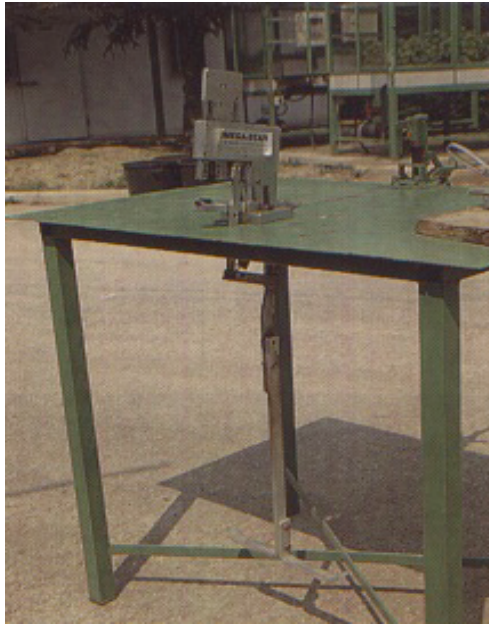
Saw type electrically powered grafting machine
