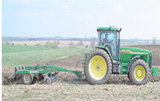
A modern John Deere 8110 Farm Tractor using a chisel plough.
