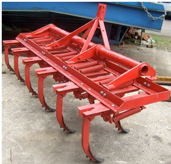
Tractor drawn cultivator- spring loaded tines
