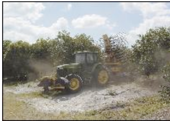
Citrus harvester Tractor-drawn canopy shaker (Oxbo make)
