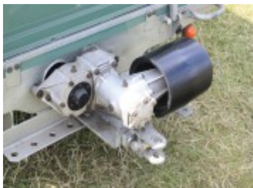
Belt pulley connected to tractor PTO
