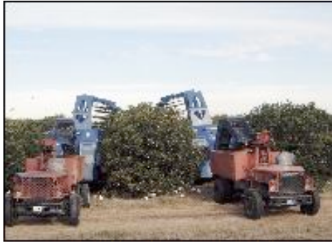
Citrus harvester -self-propelled system (Oxbo make)
