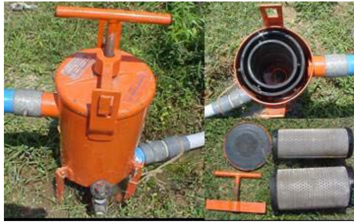
Fig.1.3 Screen filter showing steel wire mesh strainers
